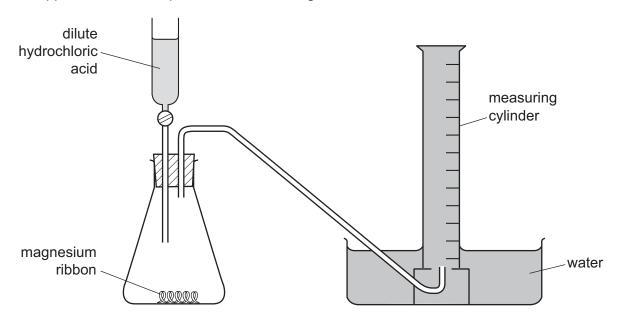
30 cm³ of dilute hydrochloric acid were added to the conical flask containing magnesium ribbon. The timer was then started and the volume of gas collected in the measuring cylinder was measured every 20 seconds for 180 seconds (3 minutes).
